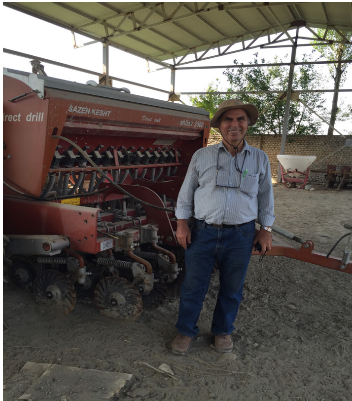
Figure 11. No-till planters are being increasingly manufactured widely; as an example, the picture shows a no-till grain drill built in Iran.
