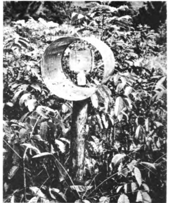
Fig. 1. 2 1/2 gallon trap used in field testing of pheromones. Note small cage, containing live H. grandella adults, suspended inside the larger can .
