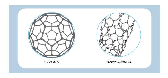
Another type of nanostructure, called "nanotube," is being manufactured as the building block of new, highly flexible yet extraordinarily strong carbon-based fibers. Nanotubes are hollow cylinders having diameters in the nanoscale range of 1 to 100 nm. Carbon nanotubes, one of the few nanomaterials currently being produced in large volumes, present some unique properties that include high conductivity, high molecular adsorption capacity, and high tensile strength. These
