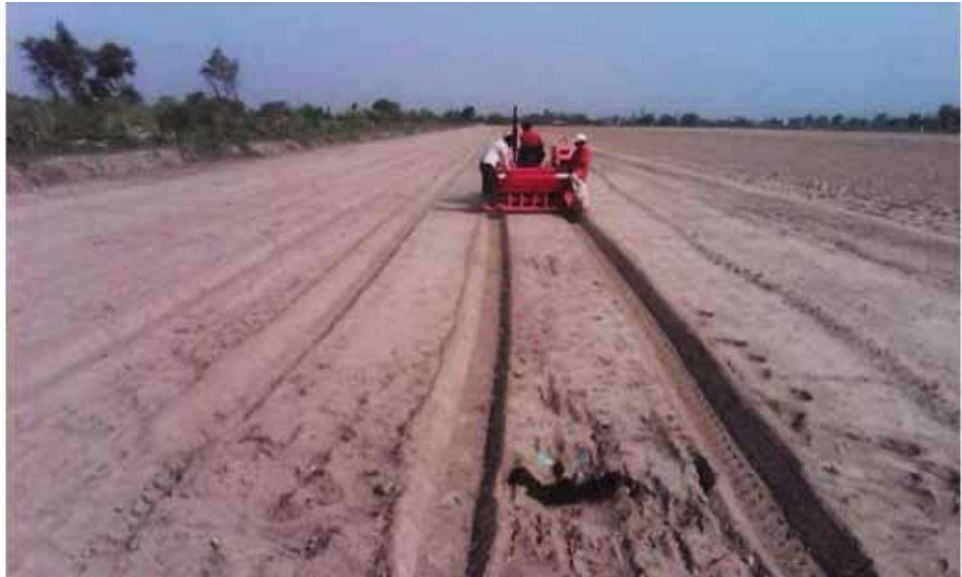
Figure 44: Machine making permanent raised beds on laser-lev- eled field, also applying fertilizer and banding compost precisely in Punjab Province of Pakistan.
