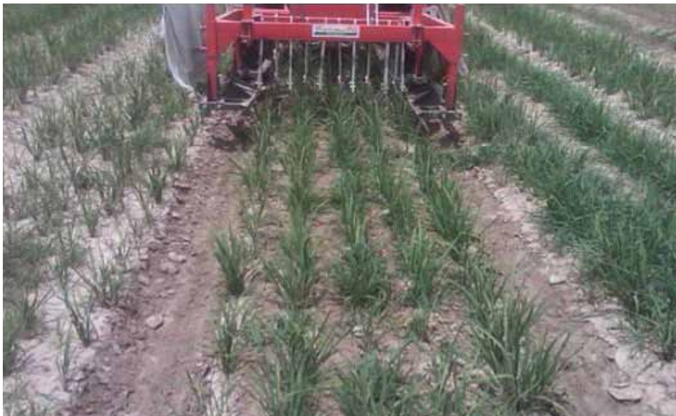
Figure 46: Weeder moving along raised beds, aerating the soil while uprooting weeds.
